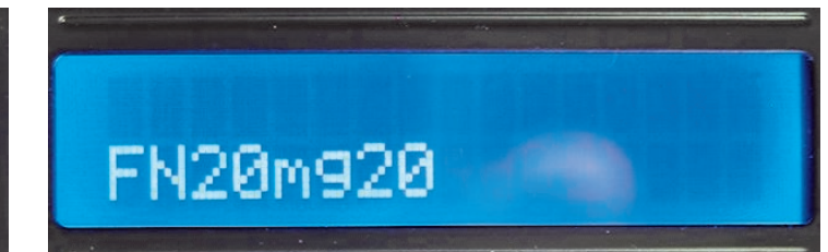
Figure 8 The 4th optional screen is new and provides your 8 digit grid square. (Looks a bit lonely compared to the other screens.)
