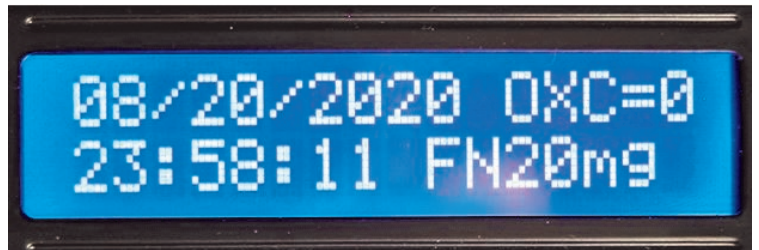
Figure 4 Default display 'B' showing the status of the 10 MHz crystal
