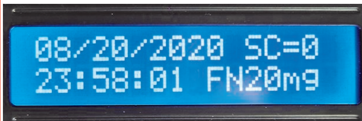
Figure 5 Default display 'C' showing the status of the self-survey - it has recently been surveyed and will count down to a zero
