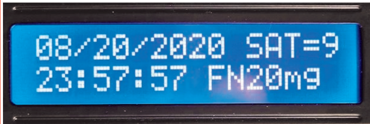
Figure 3 Default screen 'A' showing DATE, TIME, Your six digit grid
