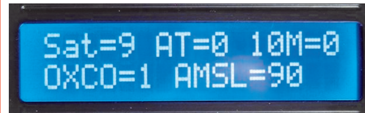
Figure 7 Useful display selected - here you get the Altitude of the GPS antenna in meters, useful with the new mapping feature when using the K1RZ/W3SZ database.
